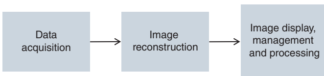
Figure 1.3 The three major stages of CT imaging, namely data acquisition, image reconstruction, and image management and processing.
