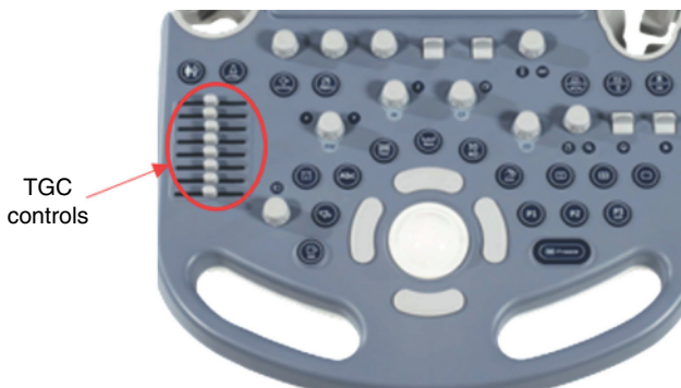
Figure 1.10 The typical time gain compensation (TGC) slide controls for different gains at different depths.
