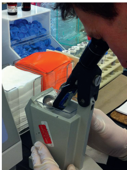
Figure 1.4 Refractometer measurement. The proportion of solids in a fluid sample is calculated by a refractometer. This value is read by looking through the eyepiece of the instrument and adjusting the eyepiece to fine focus the scale present in the refractometer.
