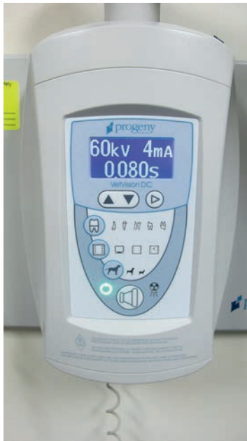
Figure 1.12 Image of a standard radiographic generator. There are three controls that can be adjusted: milliamperes (mA), kilovoltage peak (kVp), and exposure time.
