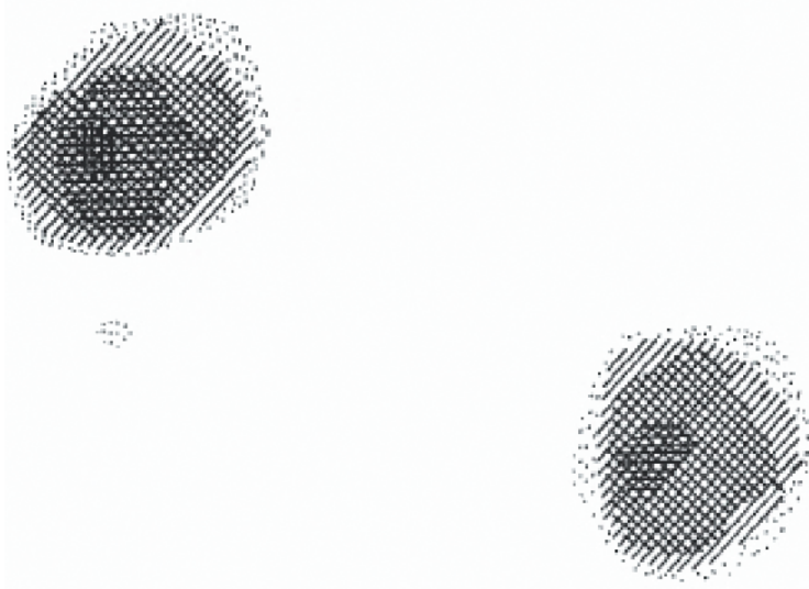
Figure 1.5 The first proton NMR image of two tubes of \text{H}_2\text{O} , which was produced by P.C. Lauterbur by combining four projections taken from different angles from his setup on a Varian A-60 spectrometer, which is currently on display at the State University of New York at Stony Brook. Source: Reproduced with permission from Lauterbur [15].
