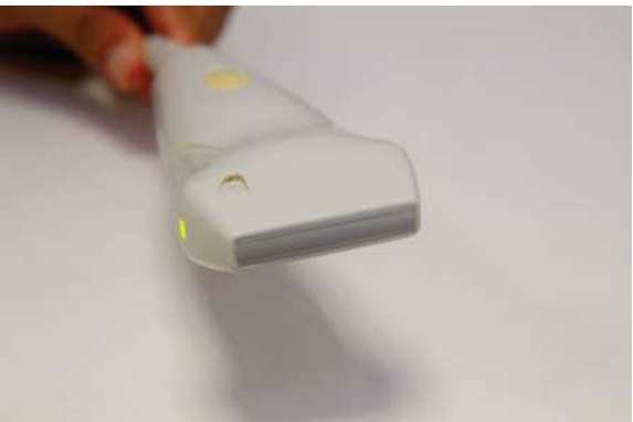
Figure 1.13 The linear probe.
