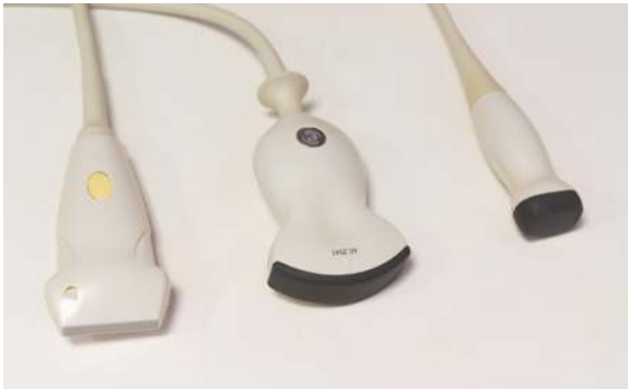
Figure 1.11 Commonly used ultrasound probes. From left to right: high frequency linear probe; curvilinear probe; phased array probe.
