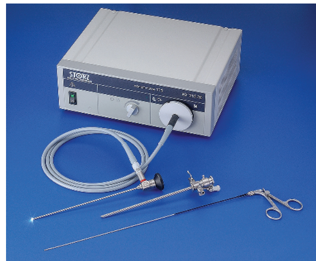
Figure 1.9 The light transmission system for a rigid endoscopic telescope with the large external remote "cold light source" shown as a box, the flexible fiberoptic light cable seen as a coiled gray cord attached to the light source on one end, attached to the light guide post of a telescope at the other end, and there is a fiberoptic light guide bundle in the rigid telescope continuing from the light post through the telescope shaft to conduct light to the tip of endoscope. This light transmission system is composed of incoherent fiber bundles. The image of rigid telescopes is transmitted through a series of solid glass lenses. (Source: Photo courtesy of Karl Storz; ©Karl Storz SE & Co KG, Germany.)
