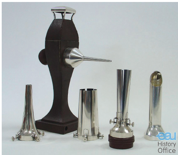
Figure 1.1 The first rigid endoscope, built by Bozzini in the early 1800s. The light source was a candle directed by a mirror into a metal tube. (Source: Downloaded from the European Museum of Urology Website.)
