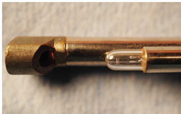
Figure 1.2 A major step in advancing technology or endoscope development was placing the exposed wire filament in an enclosed bulb. This improved the quantity of light and decreased the risk of tissue burning. This picture is of a standard endoscope bulb connected to an ACMI 120° cystoscope. The bulb is 4 mm long and 2 mm wide.
