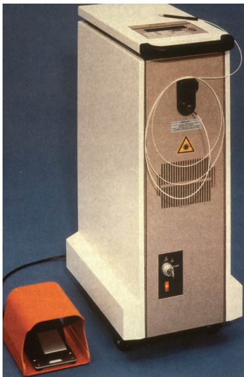
Figure 1.22 Nd:YAG laser device (American Dental Technologies, Southfield, MI, USA). Source: Dr. Georgios E. Romanos
