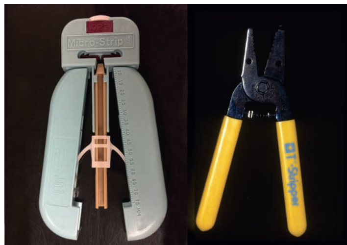
Figure 1.17 Special tools to remove plastic coating around glass fiber without damaging the fiberoptic. Source: Dr. Georgios E Romanos.
