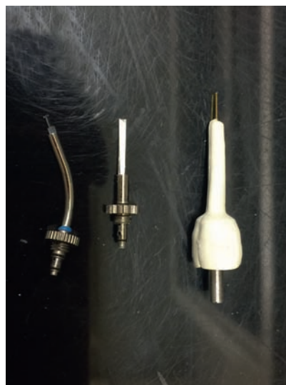
Figures 1.12–1.14 Special tips for direct connection with the hand piece (left) for Er:YAG laser made by sapphire or glass fiber for Er:YAG or diode lasers (middle) and for Er,Cr:YSGG laser (right). Source: Dr. Georgios E Romanos.
