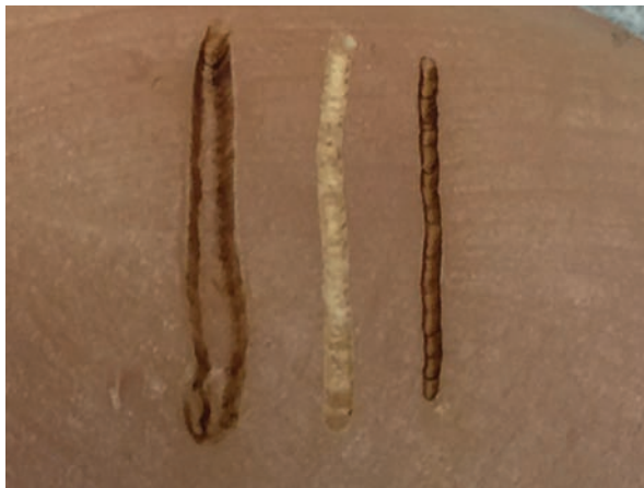
Figure 1.32 Comparative incisions using blue laser light (left), pulsed CO 2 laser with microsecond pulses (middle, char-free), and CO 2 laser (continuous wave and average power of 2 W (continuous wave) in chicken breast showing minimal carbonization zone but sufficient incision depth. Source: Dr. Georgios E. Romanos.
