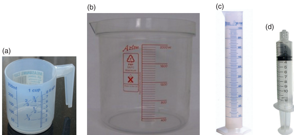
FIGURE 1.4 Measuring devices: (a) measuring cup – 250 mL; (b) large beaker – 2000 mL; (c) graduated cylinder – 1000 mL; (d) syringe – 12 mL.
