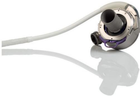
Fig. 1.3 The HeartMate 3, like the HeartWare left ventricular assist device, is a centrifugal pump but, rather than using bearings, has a fully magnetically levitated (Full MagLev) rotor. (Courtesy of Abbot Laboratories, Lake Bluff, IL.)
