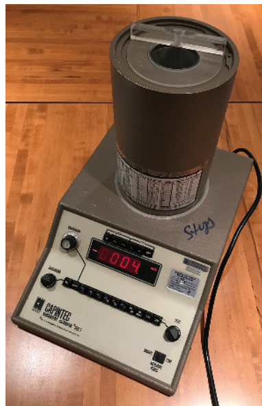
Figure 1.56 Well-type ionization chamber and electrometer (isotope calibrator) used to measure the activity of a radioactive sample before administration of the sample to a patient. The volume of the sample to be administered is computed from the measured activity, often automatically by the isotope calibrator.
