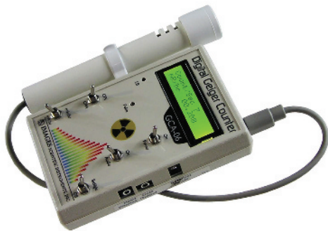
Figure 1.60 Portable survey meter equipped with an end-window G-M tube.
