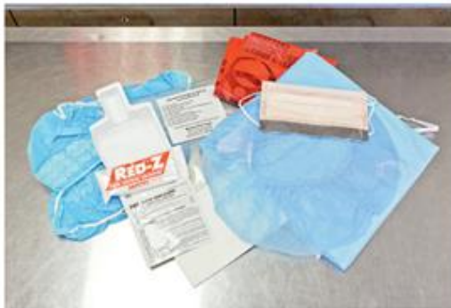
Fig. 1.2 Spill Cleanup Kit. These kits generally contain biohazard bags, personal protective equipment, absorbent materials, and disinfectants.
