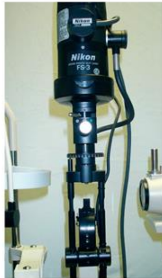
Fig. 1.4 Illumination system of a slit lamp biomicroscope.
