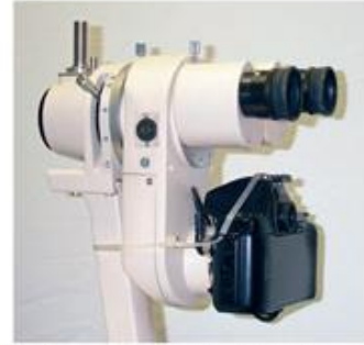
Fig. 1.5 Observation system of a slit lamp biomicroscope.
