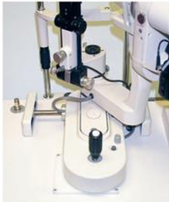
Fig. 1.3 Mechanical system of a slit lamp biomicroscope.
