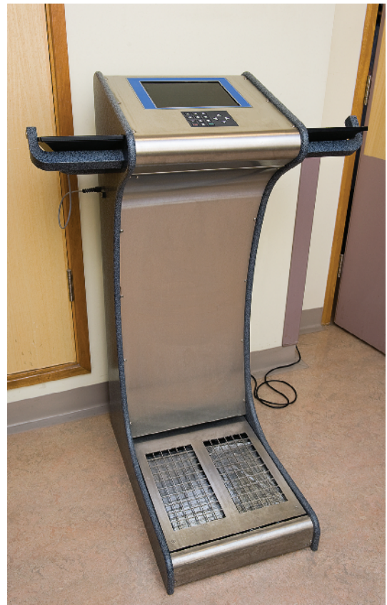
Figure 1.6 Hand and foot radiation monitor. Source: Dougherty and Lister (2011).
