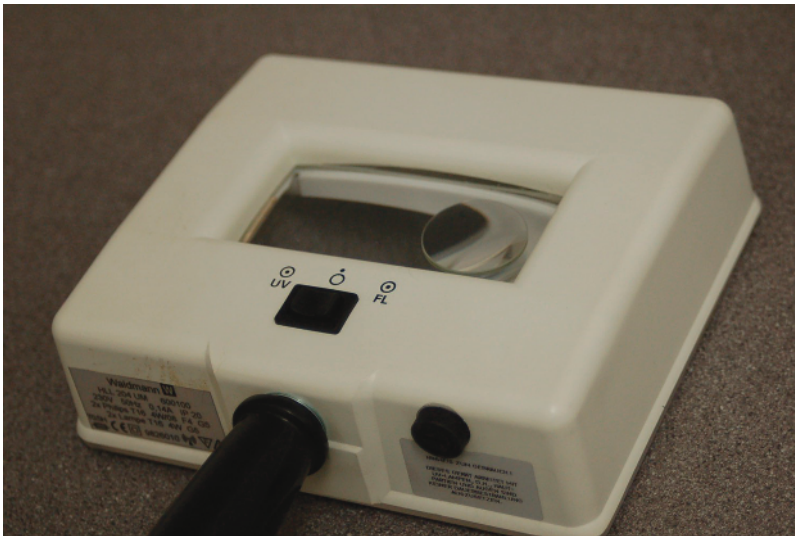
Figure 1.2 A magnifying lens with illumination. In this case the lamp doubles up as a Wood's lamp for dermatophyte detection.
